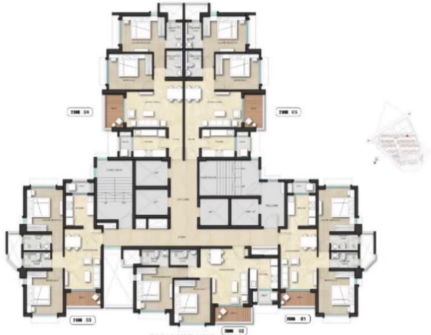
TYPICAL FLOOR PLAN (W48) (1ST - 7TH, 8TH - 12TH, 15TH - 18TH, 20TH - 23RD, 25TH - 28TH, 30TH - 33RD, 35TH - 38TH & 40TH)
